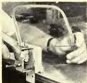
The base of the engine, like most of the wood parts, can be cut with a coping saw or power jigsaw. The engine and cars are 5" long while the coal tender is 3 1/2".
