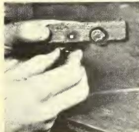
Checker wheels and car bases are drilled to take a 1/8" dowel stick axle. Axles are fastened to the wheels with glue. A little oil will make the wheels turn freely.
